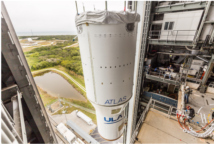
The Centaur upper stage is hoisted into the VIF to be placed atop the Atlas V rocket. Photo credit: United Launch Alliance.
