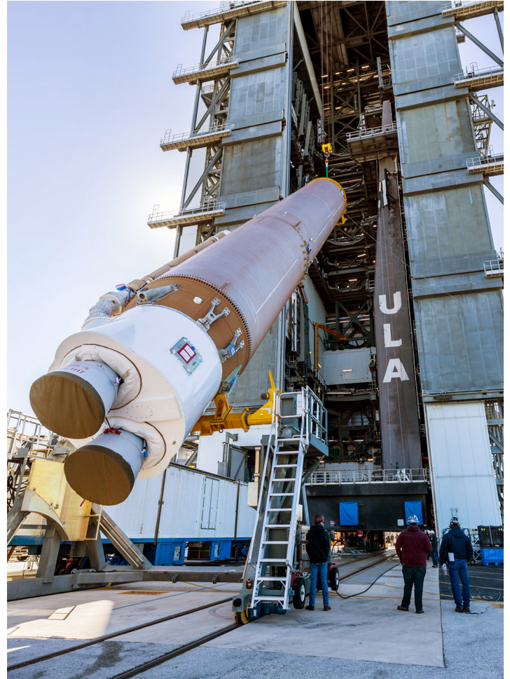
The GOES-T Atlas V first stage booster lifted into position on the stand in the VIF. Photo credit: NASA/Kim Shiflett
