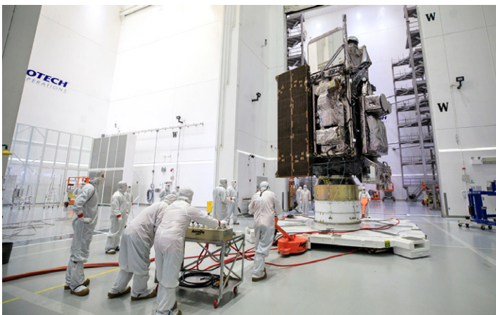
GOES-T is mated to the payload adaptor in preparation for encapsulation. Photo credit: NASA/Kim Shiflett
